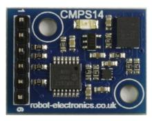
For **I2C** the mode pin can be left open or pulled to the supply voltage, for **serial mode** the mode pin should be connected to 0v ground.
