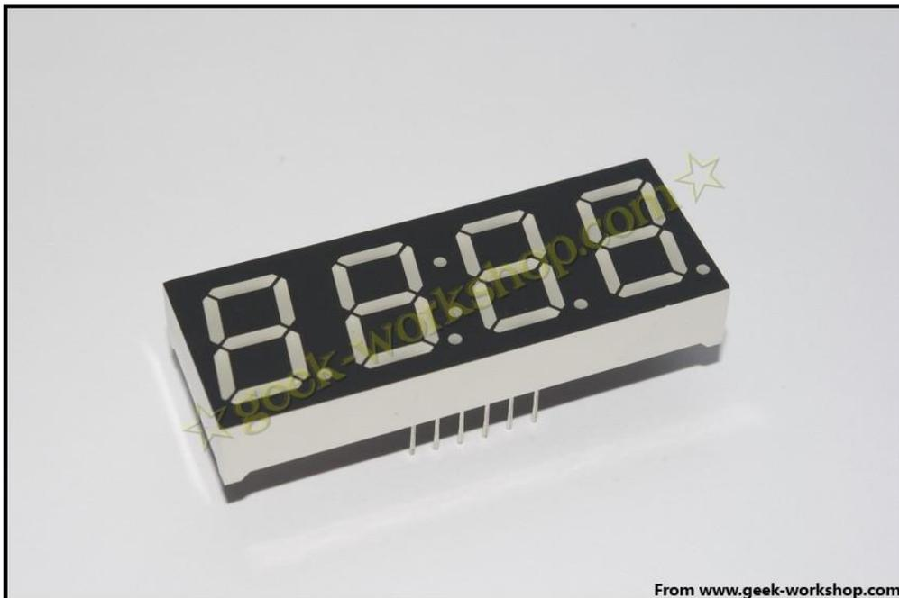
For 4-digit displays, there are 12 pins in total. When you place the decimal point downward (see below photo position), the pin on the lower left part is referred to as 1, the upper left part 12.
