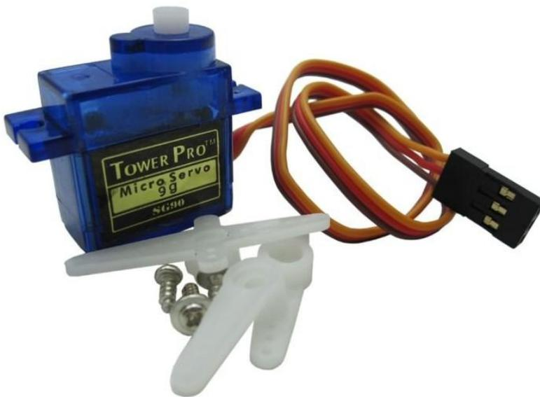
Servomotor comes with many specifications. But all of them have three connection wires, distinguished by brown, red, orange colors(different brand may have different color). Brown one is for GND, red one for power positive, orange one for signal line.
