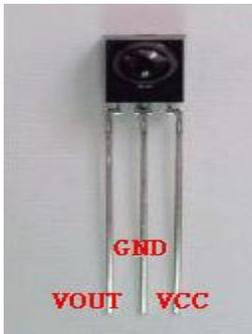
Infrared receiver has 3 pins.
